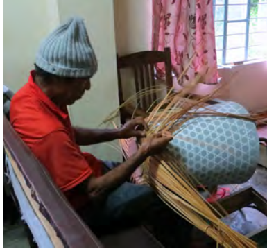
Fig. 5 Artisan weaving laundry basket by using FRP pre-patterned mold.
