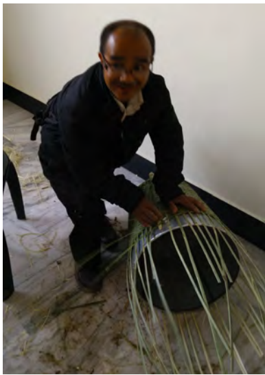
Fig.2 (Left) Artisan weaving the laundry basket using green outer sheath of bamboo as slivers
