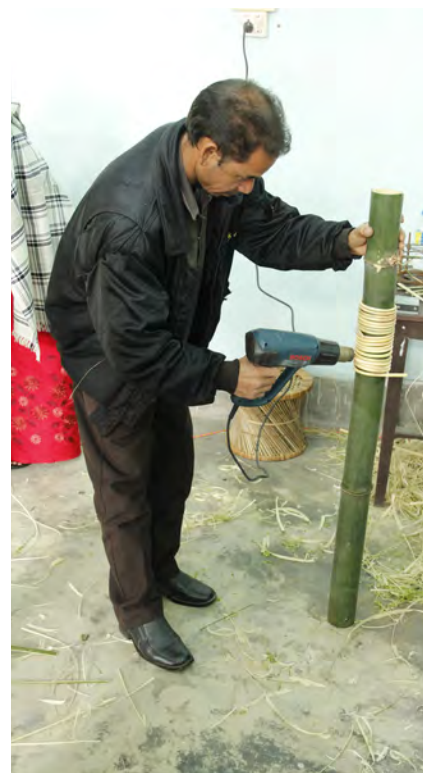
Fig.10 (Left) Heat bending of cane for base of waste paper bin.
