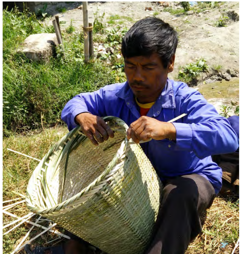
Fig.3 (Right) Artisan closing the rim of the laundry basket by interlocking of the slivers
