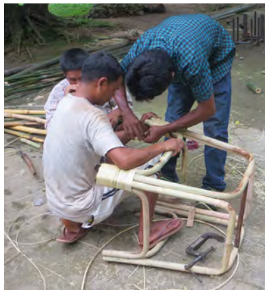
Fig. 8 (Below Right) Bending of cane by using mold.
