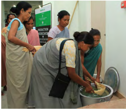
Fig. 3,4 & 5 Demonstration of bamboo processing techniques by chemicals – boiling, washing and soaking bamboo slivers.
