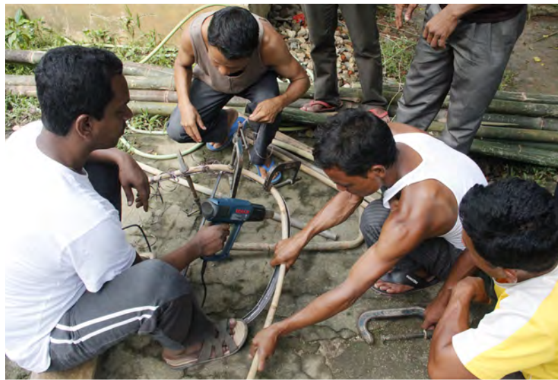
Fig. 6 (Right) Mr. Subrato guiding artisans for proper bending of cane by using mold.
