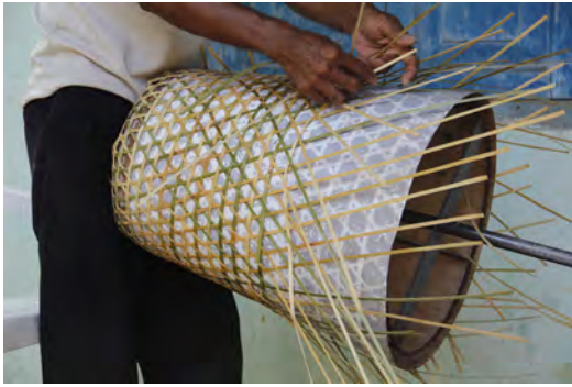
Fig. 4 Laundry basket weaving on pre-patterned mold.
