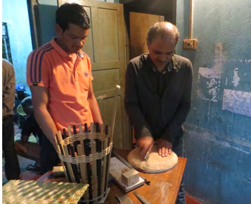
Fig. 5 Artisan weaving laundry basket by using FRP pre-patterned mold.
