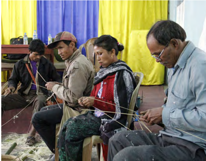
Fig.5 (Right) Artisans preparing bamboo slivers for Laundry basket
