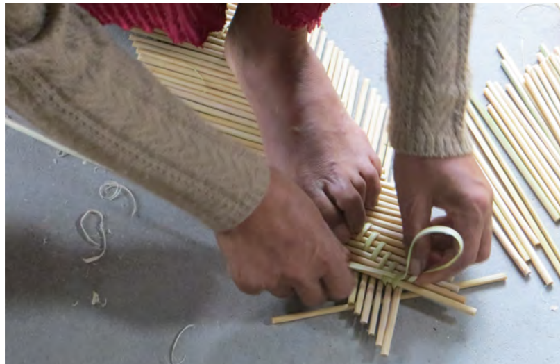
Fig. 6A Artisan arranging sticks to form straight band of them.
