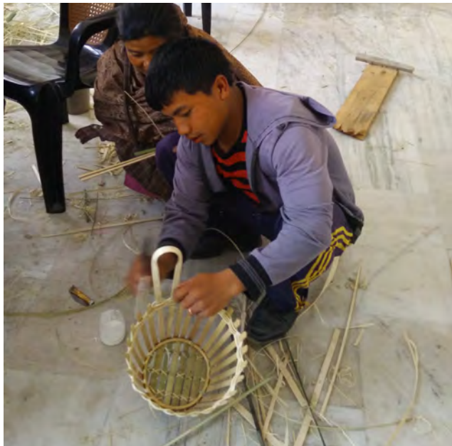
Fig.6 Artisan finishing the paper basket
