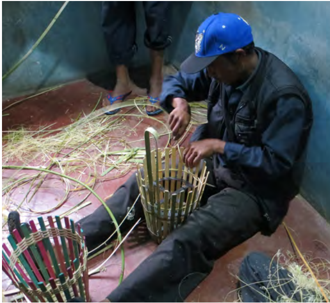
Fig. 3 Artisan finishing first waste paper bin by using mold.
