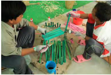
Fig. 12 Coloring bamboo strips by using potassium permanganate.
